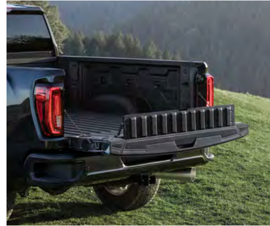
PRIMARY GATE LOAD STOP With the primary gate open, the load stop can help prevent items from sliding out of the bed.
